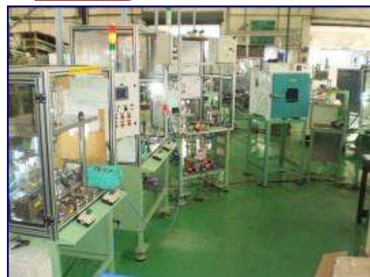
➤ Dedicated Thermostat Cooling Module Assembly Line
